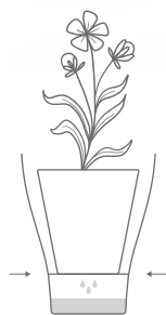
water reserve system
