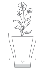
water reserve system
